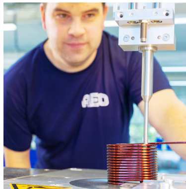
Efficient cooling thanks to single layer design for REO EDGE-WINDING
